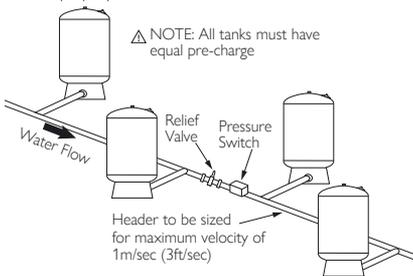
Fig. 1.5 Multi-tank Installation
